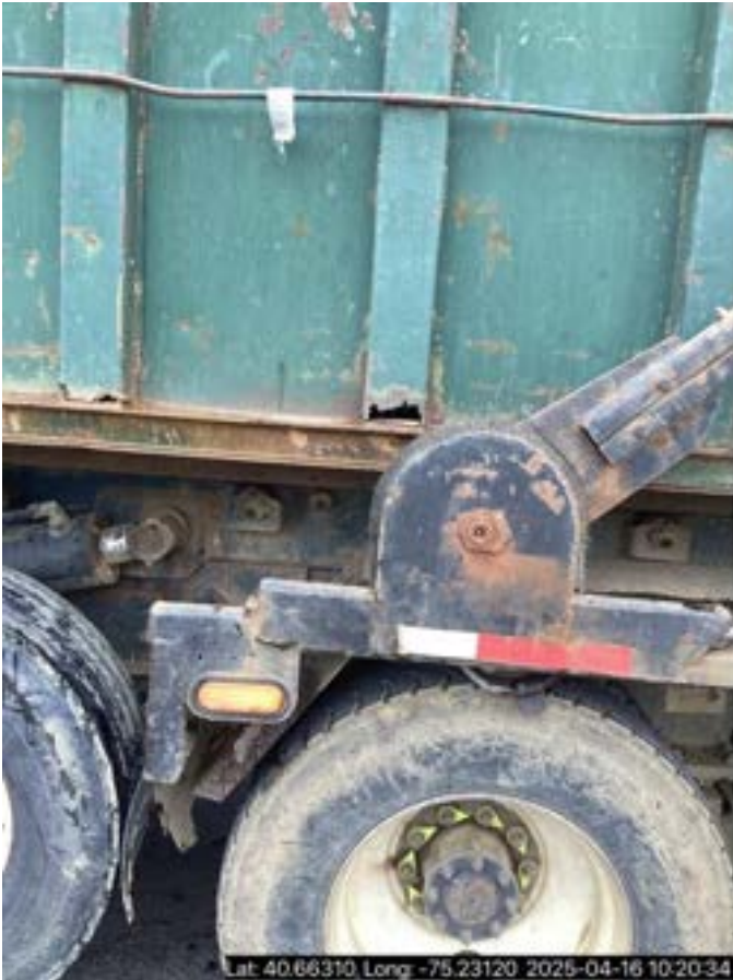
Photo #1- Leak observed on roll off container
