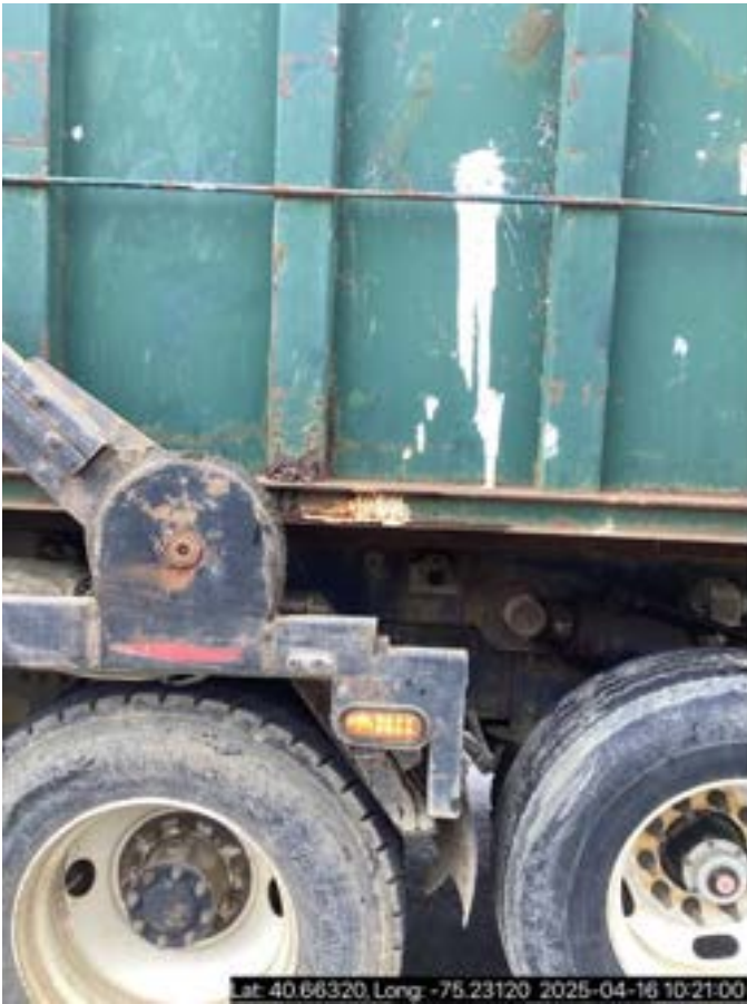
Photo #3- Damaged side of vehicle with leak observed on roll off container
